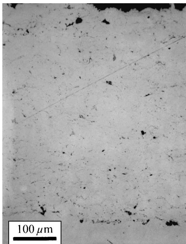
Fig. 10 Micrograph of a PPS stainless-steel coating
